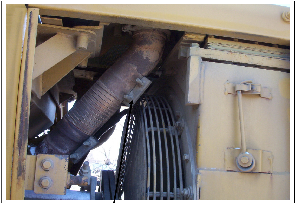
This may have to be loosened and rotated out of the way to install the condenser.
