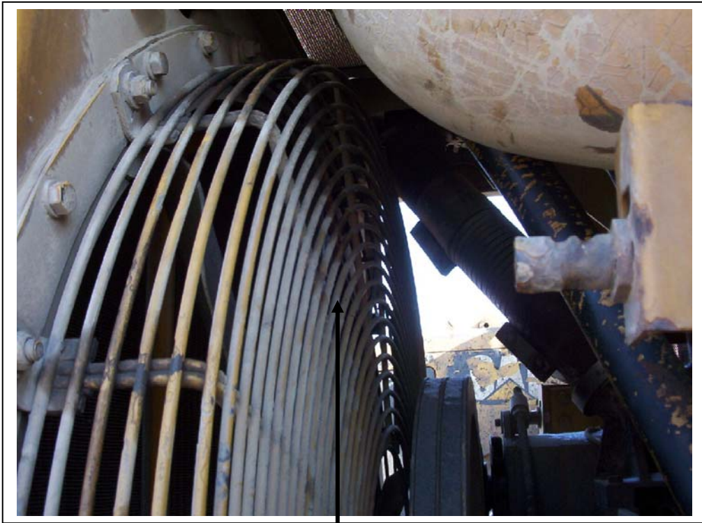
Condenser will mount here in front of the pulley.
