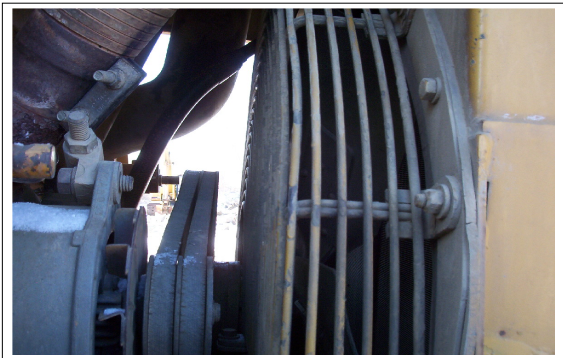
Condenser mounts to fan screen (see page 11) between pulley and screen. Mount as low to hub as possible with #6 (smaller) fitting at bottom.
